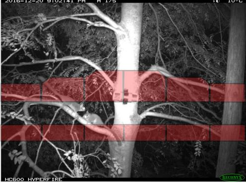
Examples of LBP camera alignment with bait stations and the location of the Reconyx PIR sensor
