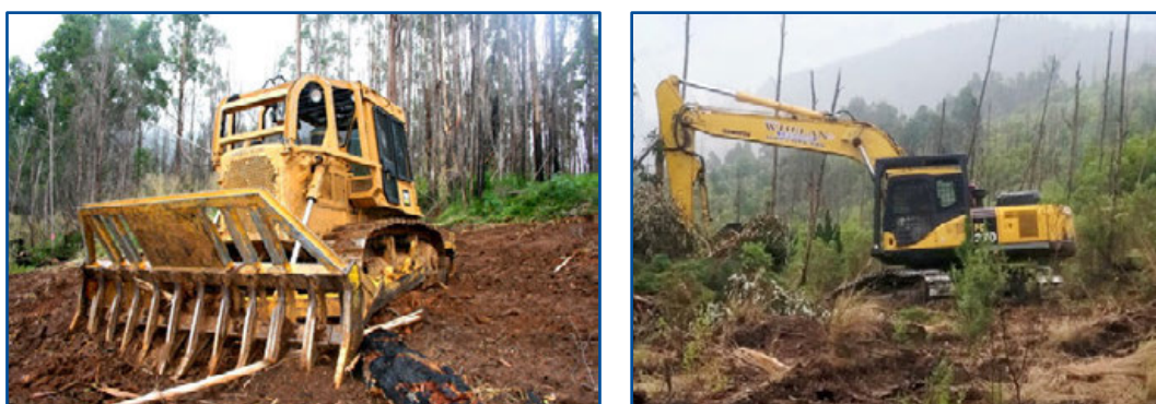
Figure 86. (Left) Root rake fitted to a bulldozer in Ash country, and (Right) an excavator lyrebirding targeted areas amongst grasses to establish seedlings. Grasses had been previously sprayed.
