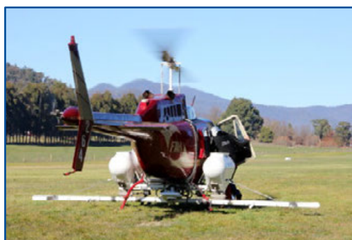
Figure 115b. Two rotary-wing aerial sowing configurations used to either sow smaller sowing operations, or the smaller shapes in large sowing operations. ( Left ) under-belly heliseeder spinner system with internal seed hopper (Paton Air Helicopters). ( Right ) An air-blown delivery system with external hoppers (Forest Air Helicopters).
