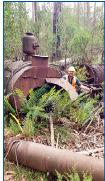
Figure 12. (Left) Peter Fagg in 2016 inspecting a preserved winch known as “The Washington” which was part of a high-lead logging system in Alpine Ash forest on the Nunniong Road, Swifts Creek. (Right) Mick Hansby in 2020 doing the same in Alpine Ash forest along Pine Track in the Blue Range, Rubicon.
