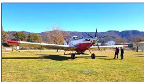
Figure 115a. The fixed-wing aerial sowing configuration used to sow larger shapes following the 2020 bushfires. Air Tractor ( left ), showing belly-mounted fertiliser unit with internal hopper, modified for Ash seed delivery at right (Pay's Air Service).
