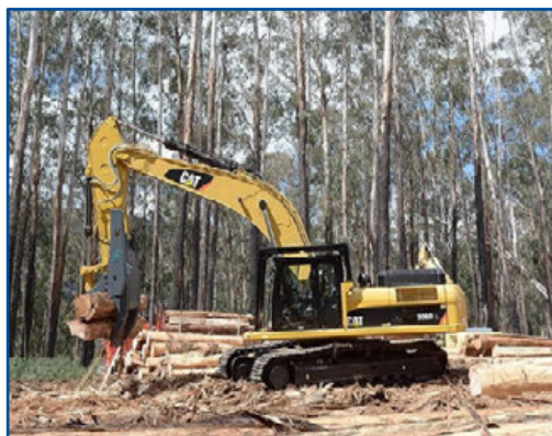
(Right) A CAT 336D excavator with a Logfork 4 grapple head with saw managing Alpine Ash logs on a landing in the Central Highlands, circa 2020 (image: Hardwood Forest Products Australia).
