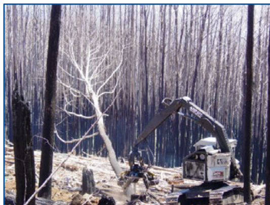
Figure 96. Mechanised harvesting is the safest and most efficient form of salvage harvesting in native forests. Here an excavator with boom-mounted falling head is processing fire-killed Alpine Ash in NE Victoria during January 2004, following the 2003 bushfires.
