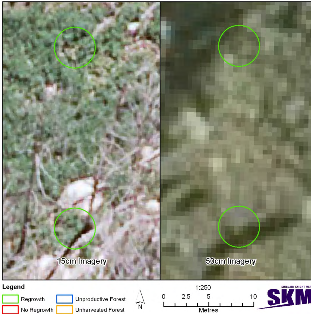
Figure 16 Comparison of 15 cm and 50 cm resolution imagery at the 1:250 scale
