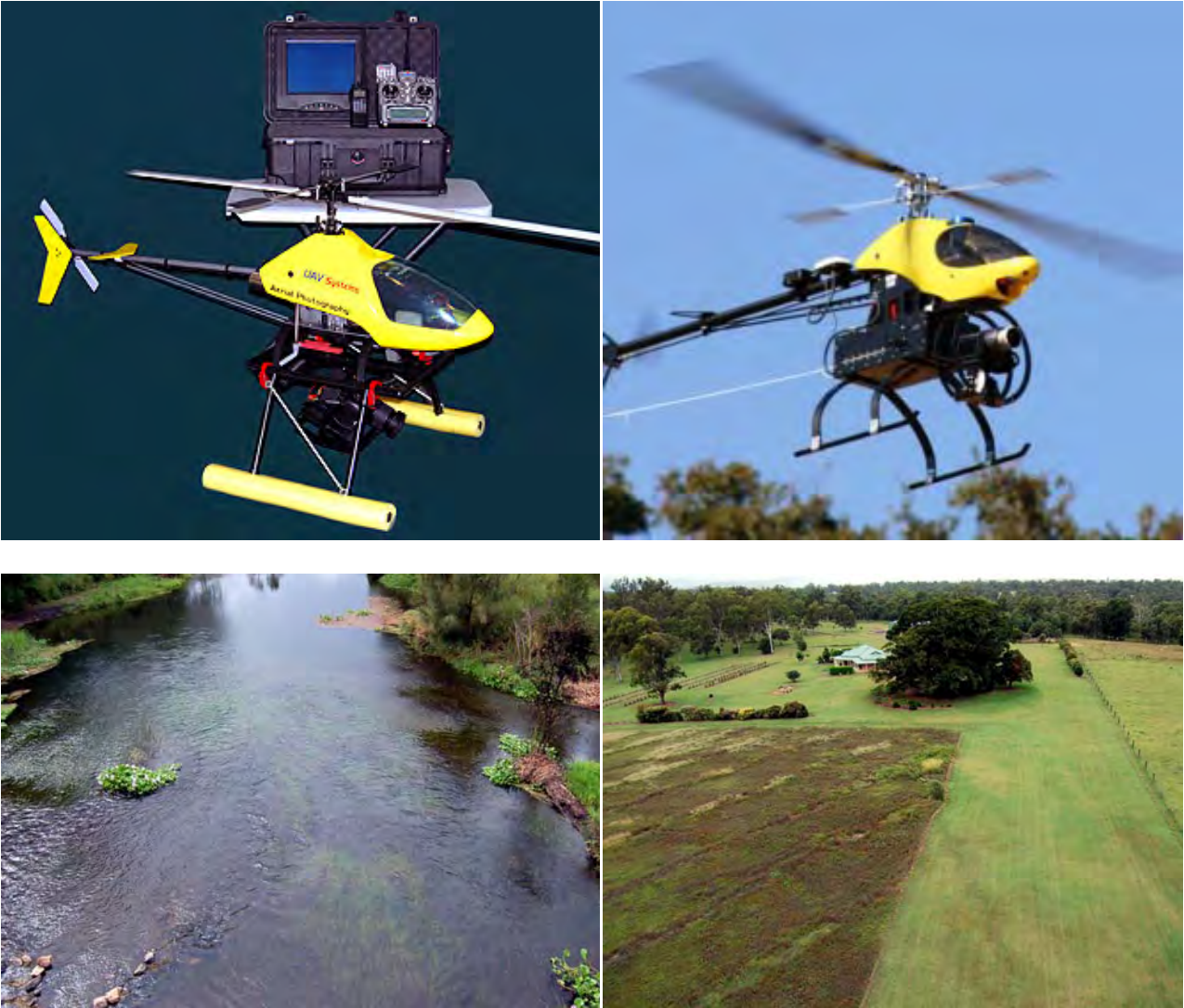
Figure 18 Rotor wing UAV (Neural Robotics inc., USA) and imagery acquired.
